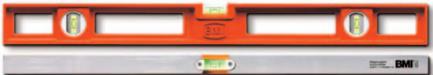
Heavy-weight aluminium die-cast level with two milled measuring surfaces. Orange powder coating. Very high torsion-resistance. Grip holes for easy handling. Also available with 2 vials (in 40 and 60 cm) as 665. Measuring accuracy in normal position 1.0 mm/m.
