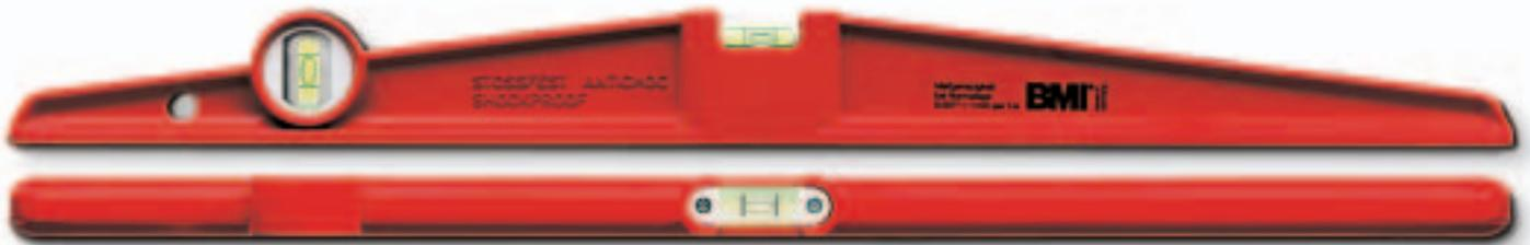
Heavy-weight, trapezoid-shaped aluminium die-cast level with milled measuring surface. Level body with orange powder coating. Very high torsion-resistance. Measuring accuracy in normal position 1.0 mm/m.
