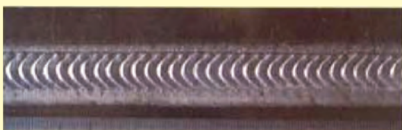
Bead - like appearance of TIG welding
