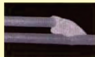
Macro cross section (material thickness 2 mm)
