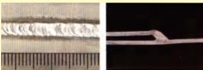
Welding process: pulsed MIG, welding current: 25 A, welding voltage: 17 V, welding speed: 70 cm/min, joint: lap fillet welding, welding wire diameter: 1,2 mm, material thickness: 0,88 mm
