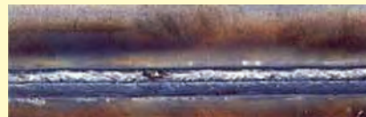
Galvanized sheet iron butt - welding
